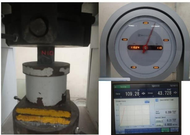
Figure 4. Test setup of CTM for compressive strength
