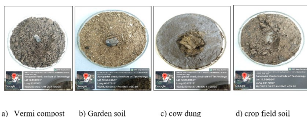
Figure 11. a-d Seventh day degradation results of cellulose based bioplastic in different soils and fertilizers
