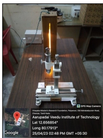
Figure 9. Measurement of thickness of bioplastics by Air Wedge Shearing Interferometer
