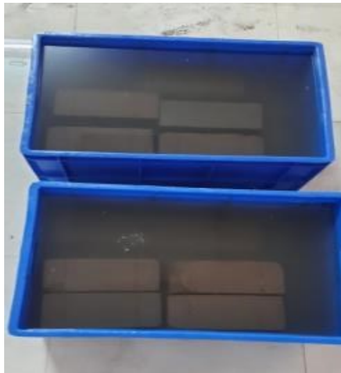
Figure 7. Chemical attack tests for solid blocks
