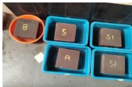
Figure 6. Experimental Setup for Initial Rate of Absorption
