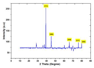
Figure 3. XRD Evaluation of biosynthesized Silver Nanoparticles from Lawsonia inermis leaf extract.
