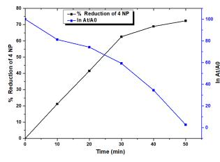
Figure 6. Rate of decrease and ln  $(A_t/A_0)$  plot of 4NP at a catalyst concentration of 0.45 mg/mL of LI-AgNPs
