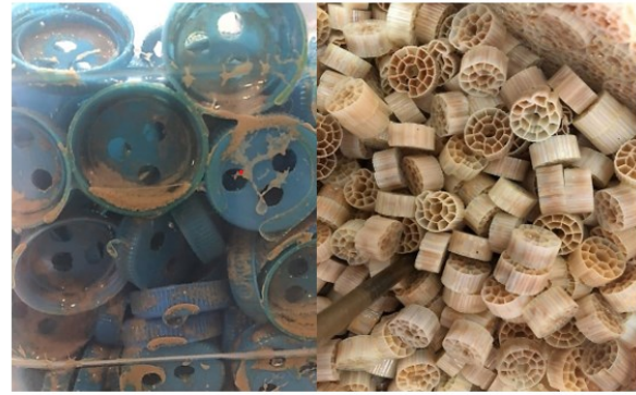
Figure 4. Observing biofilm formation during the adaptation phase
