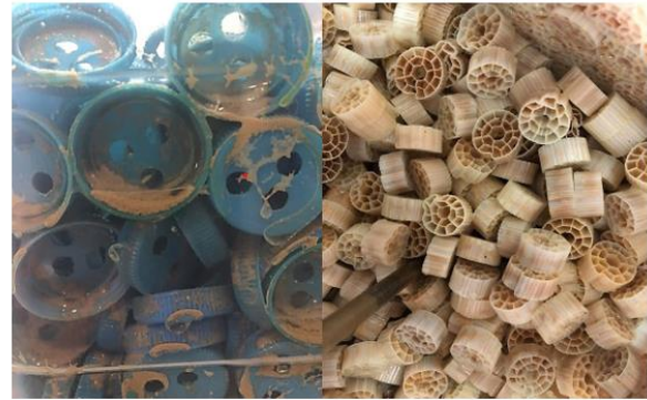
Figure 4. Observing biofilm formation during the adaptation phase
