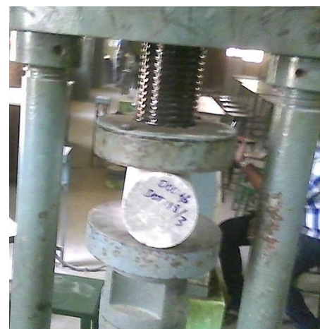
Figure 8. Testing of cylindrical specimen
