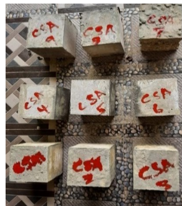
Figure 7. Concrete cubes with different percentages of CSA
