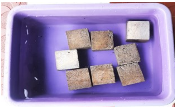
Figure 12. Test setup for water absorption
