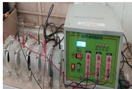
Figure 13. Test setup for RCPT
