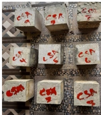
Figure 7 Concrete cubes with different percentages of CSA
