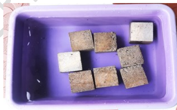
Figure 12 Test setup for water absorption
