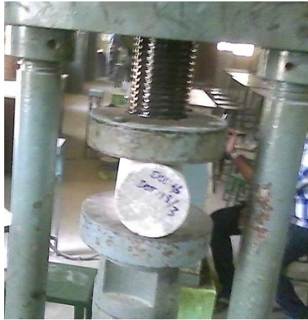
Figure 8 Testing of cylindrical specimen
