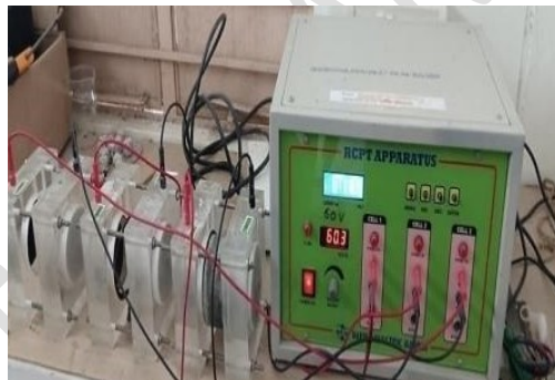
Figure 13 Test setup for RCPT
