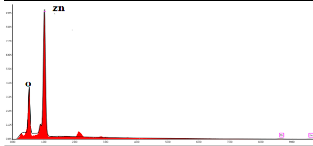
Figure8. EDS Analysis of ZnONPs
