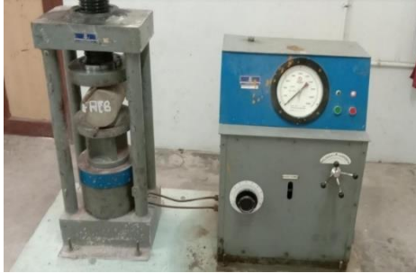
Figure 2. Split Tensile testing of a cylinder
