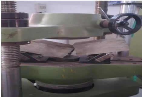
Figure 3. Flexural testing of a Prism
