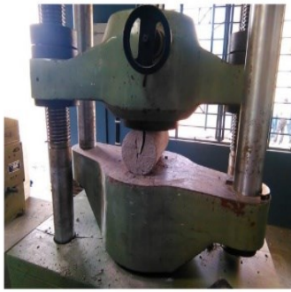
Figure 2. Split Tensile Test
