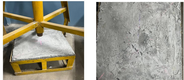
Figure 7. Impact Resistance Test (Formation of Cracks)
