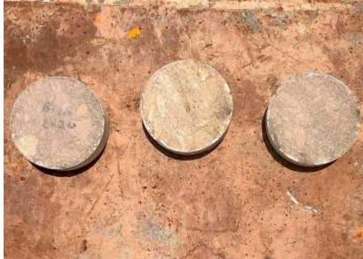
Figure. 3. Sample examined for RCPT
