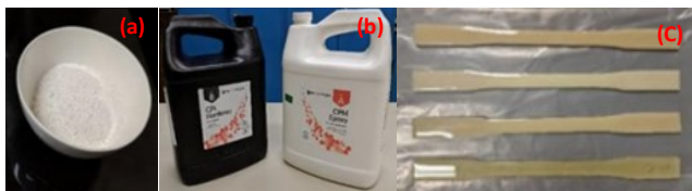
Figure 2. Sample preparation (a) Egg shell powder (b) Epoxy resin & Hardener (c) Composites
