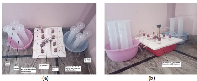
Figure 3. Biogas production set-up (a) Top View and (b) Side View
