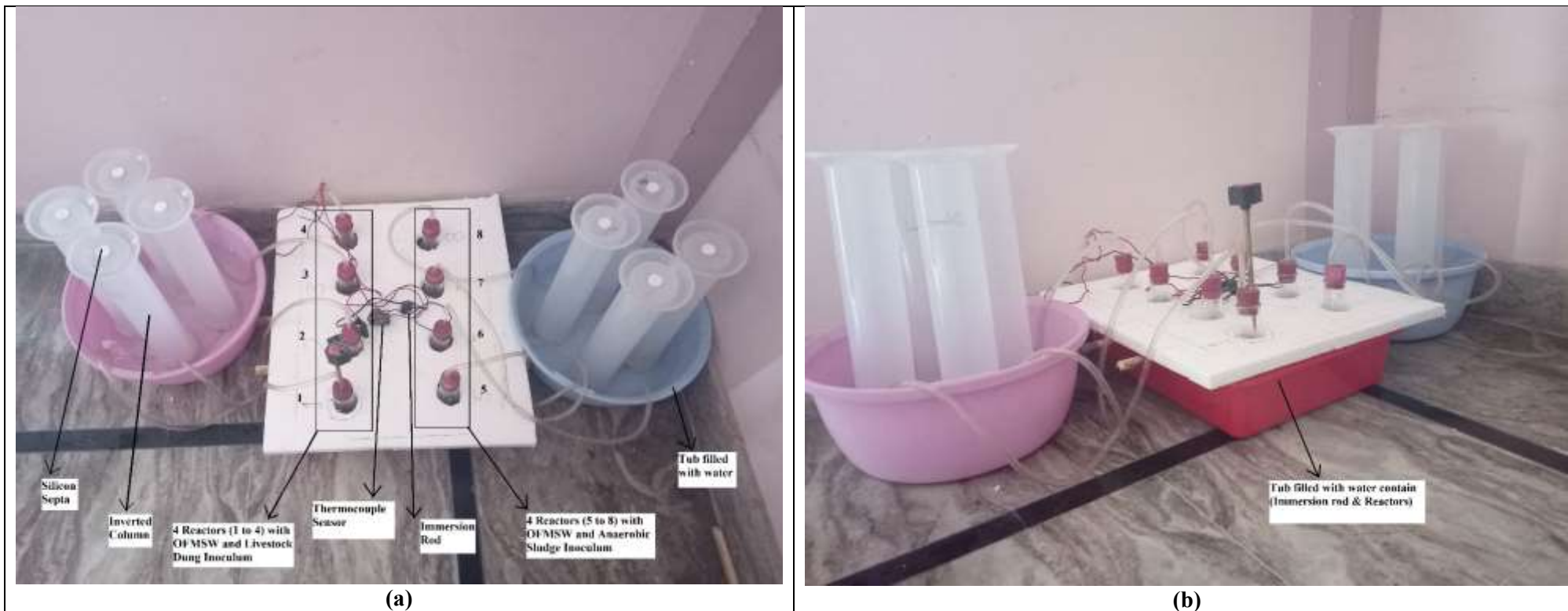
Fig 3. Biogas production set-up (a) Top View and (b) Side View
