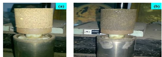
Figure 1. Standard sand specimen preparation (Figure 1: a 80:20, silica sand: cupola slag sample; and Figure 1: b 20:80, silica sand: cupola slag sample)
