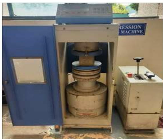
Figure 6. Specimen testing in compression testing machine
