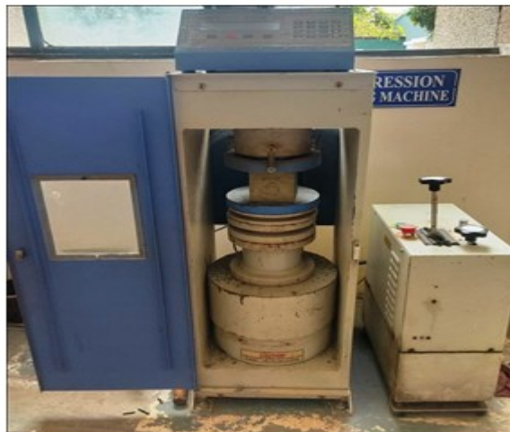
Figure 6. Specimen testing in compression testing machine
