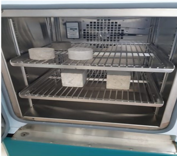
Figure 5. Specimens placed in carbonation chamber
