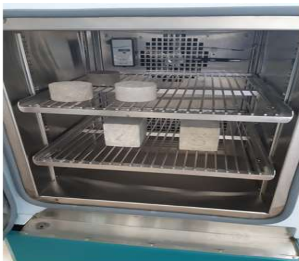
Figure 5. Specimens placed in carbonation chamber
