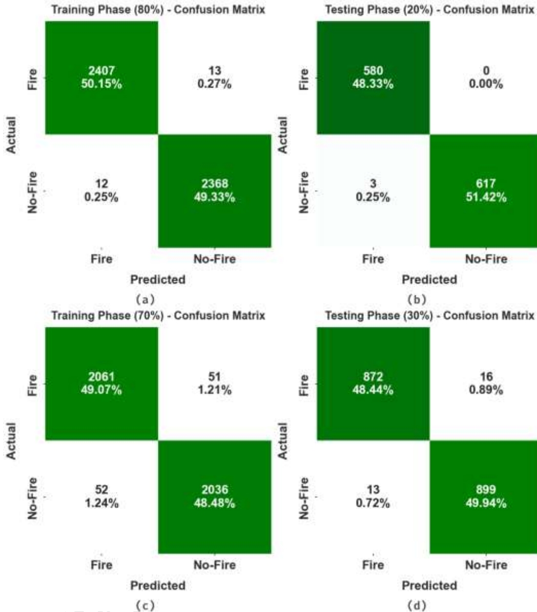
Figure 3: Confusion matrices of FFDMDL-DI technique (a-b) TRS/TSS of 80:20 and (c-d) TRS /TSS of 70:30
