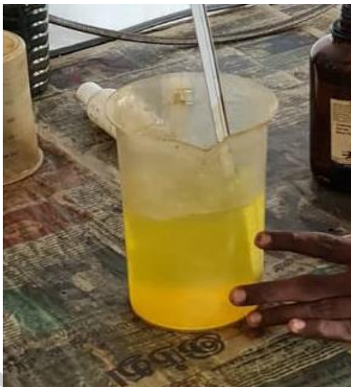
Figure 2. Diesel, Propanol and Cotton seed Oil blend
