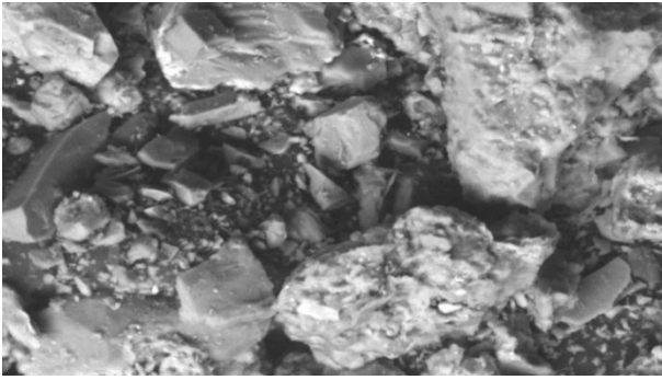
Figure 4. SEM analysis of Annona reticulata – Chitosan adsorbent
