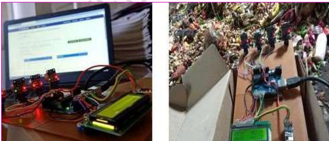
Figure 1b. IOT based gaseous emission monitoring device in the investigating area of MSW
