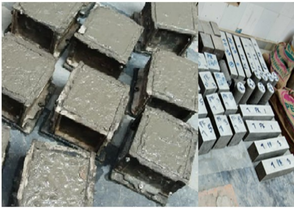
Figure 4. Casting of Specimens
