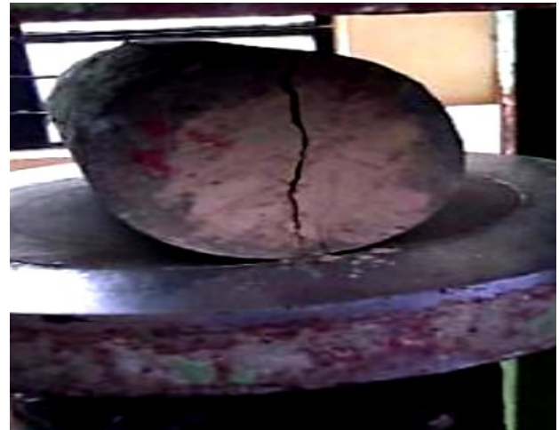
Figure 7. Crack pattern of cylinder specimen.
