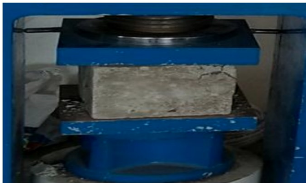
Figure 5. Compressive Strength Experimental Setup.
