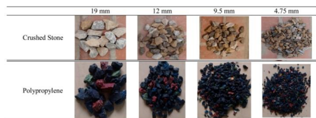
Figure 2. Coarse aggregate: (a) crushed stone aggregate (SA), (b) polypropylene (PP) aggregate
