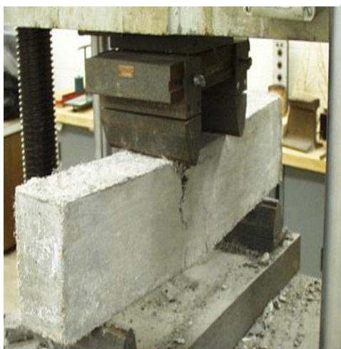
Figure 5. Flexural strength test
