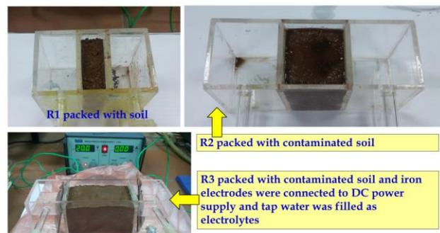
Figure 3. Distance between electrodes on electrokinetic remediation
