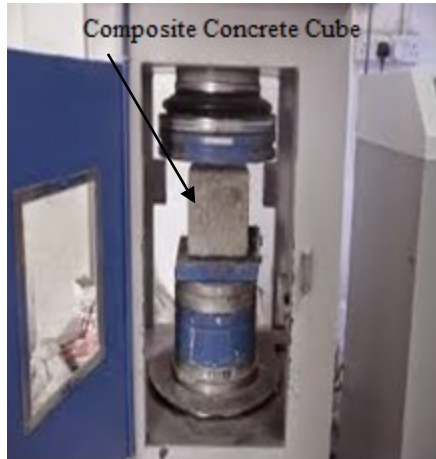
Figure 5 Compressive strength of Composite concrete by UTM
