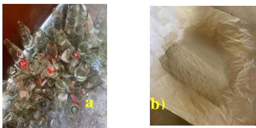
137 138 139 140 Fig. 2 a) Waste glass bottles b) Waste glass powder that passes through a 75 \mu m sieve
