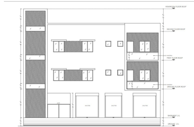
Figure 2. Elevation plan of the building.
