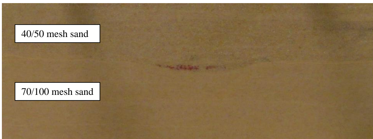
Figure 1. Image of DNAPL mixture initial distribution for the first configuration. The matrix was composed of 40/50 mesh sand. The bottom was composed of 70/100 mesh sand (Experiment 1 with 5% Tween 80)
