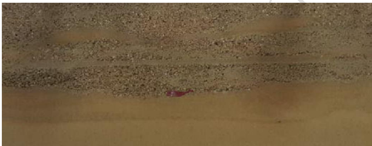
Figure 2. Image of DNAPL mixture initial distribution for the second configuration. The matrix was composed of calcareous soil and the bottom was composed of <200 mesh soil (Experiment 1 with 5% Tween 80)
