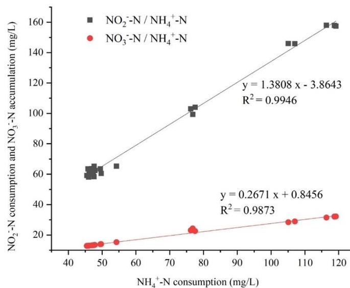
249 **Figure 3.** Fitting of stoichiometric number changes during reactor operation
