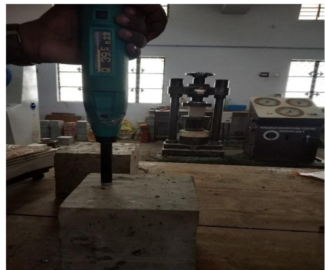
Figure 7. Rebound Hammer test
