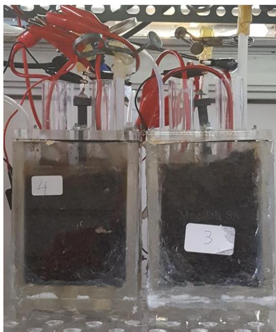
**Figure 1.** Photo of the two identical MFC units
