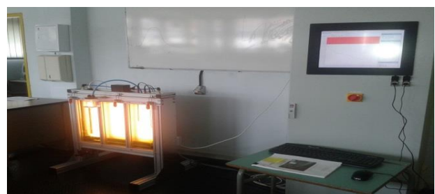
Figure 1. The 25 L laboratory flat plate photobioreactor
