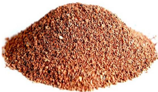
Figure 2. Mixture of sand with nanoparticles of Fe 2 O 3
