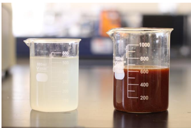
Figure 3. Treated sample after using a mixture of ferric nanoparticles and sand (left after treatment, right original sample)
