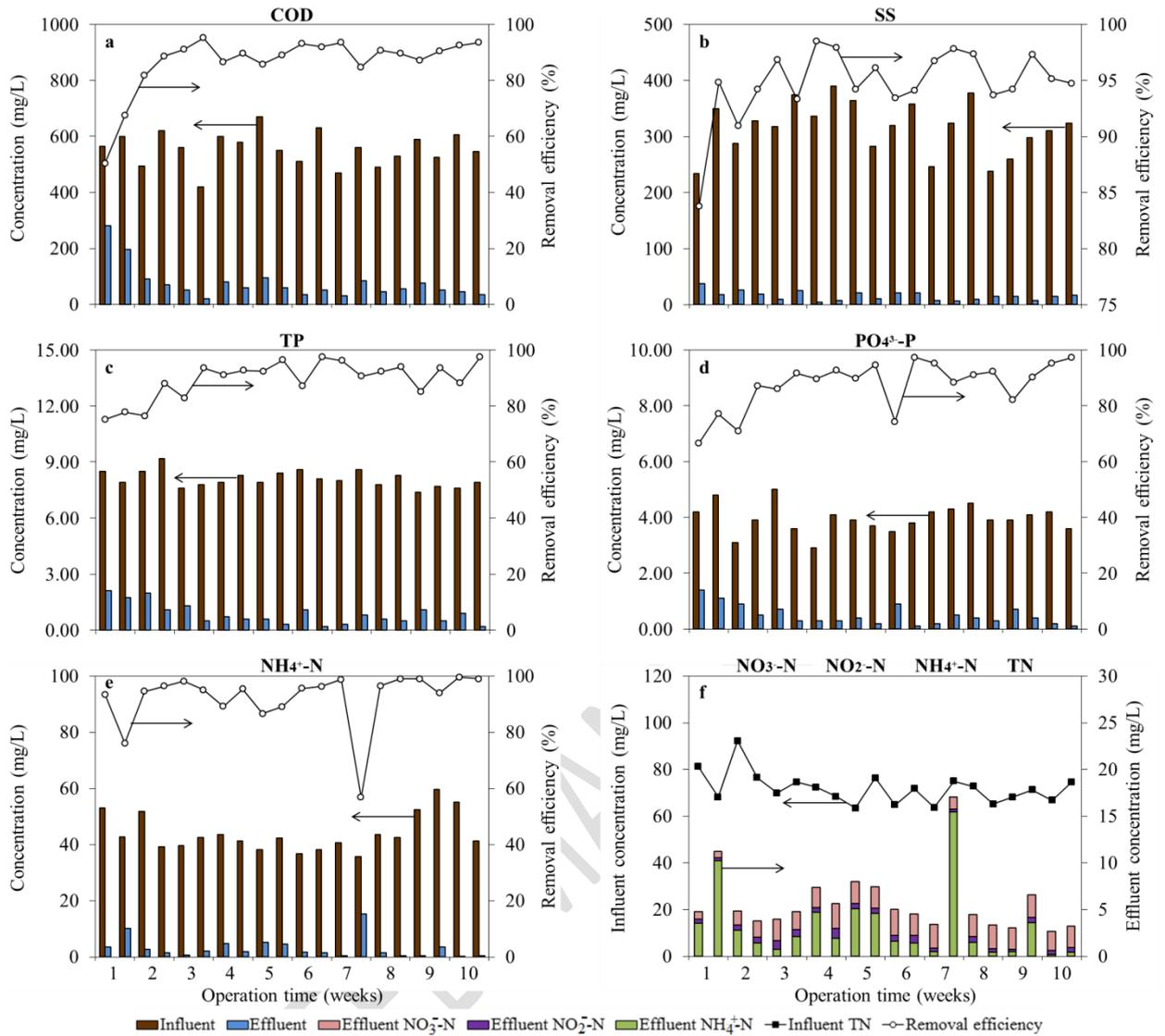
**Figure 2.** The change of influent and effluent concentrations along with removal efficiencies for (a) COD, (b) SS, (c) TP, (d) PO<sub>4</sub><sup>3--</sup>P, (e) NH<sub>4</sub><sup>+</sup>-N, (f) TN, NO<sub>3</sub><sup>-</sup>-N, and NO<sub>2</sub><sup>-</sup>-N
